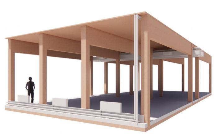
AXON OF MECHANICAL SYSTEM SHOWING JAGA UNITS AND PIPING
